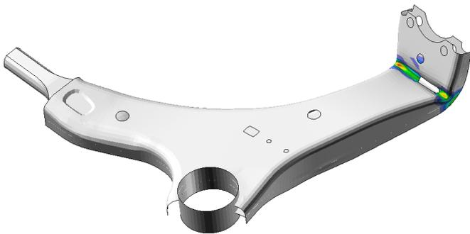
Elasto-plastic simulation of an automotive link arm
