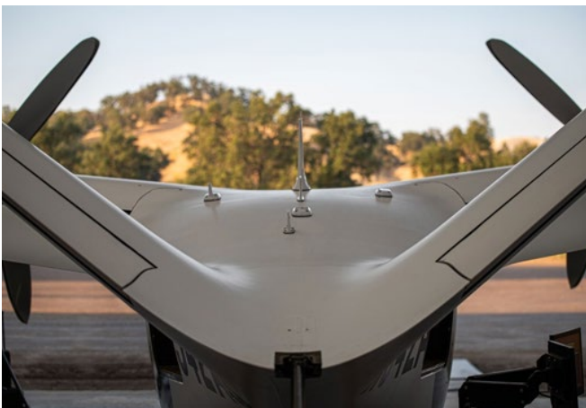
Above: Rear image of Joby’s eVTOL aircraft, showing the vast amounts of doubly-curved surfaces on the fuselage and wing
