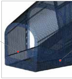
Engineers de-featured complex surface facets (curves when meshing)
