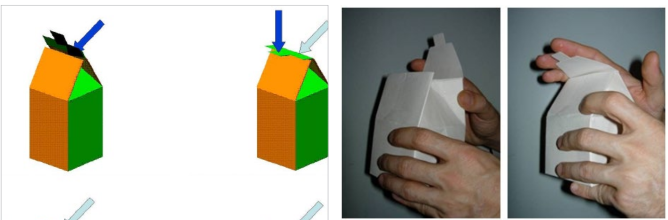
Figure 2. Tuck-in operation by human fingertip and kinematic analysis. From top left to the bottom right: a) first flap folding, b) second flap folding, c) the third flap folding, d) the tuck-in of the third flap.
