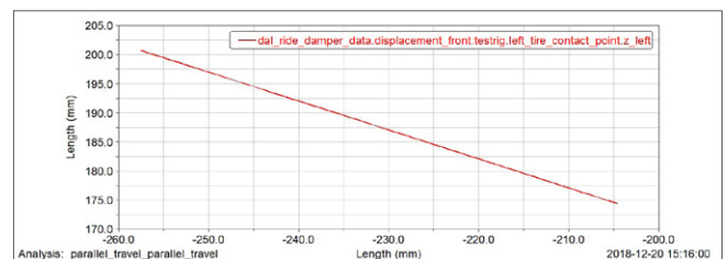
Spring stroke: The postprocessing plot shows the desired linear relation between spring deflection at the wheel and spring stroke
