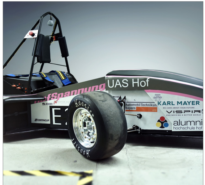
Bonnie: The fourth generation of the fast electric cars from Hof comes with 30 percent weight reduction and accelerates to 100 km / h in 3.5 seconds
