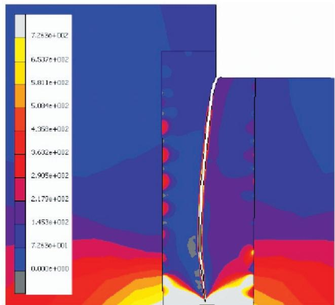
Predicted crack growth paths for notched cylinder, where the crack grows from the outer diameter.
