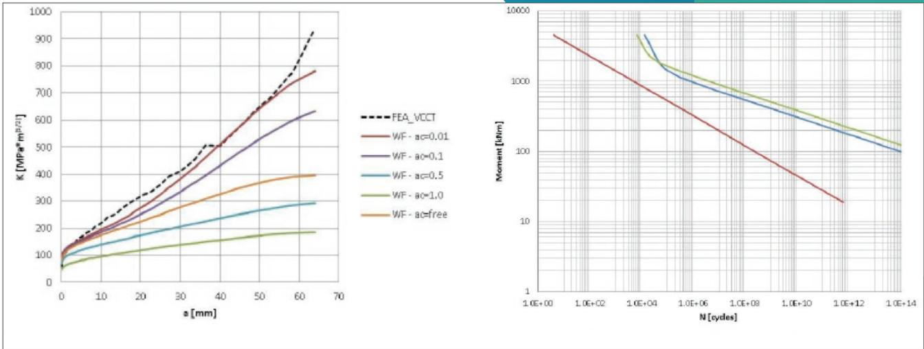
Crack growth approach, with weighing function and VCCT method, shows longer life for cylinder with notch. In the curve on the right, both crack growth and S-N results are plotted in an S-N diagram.
