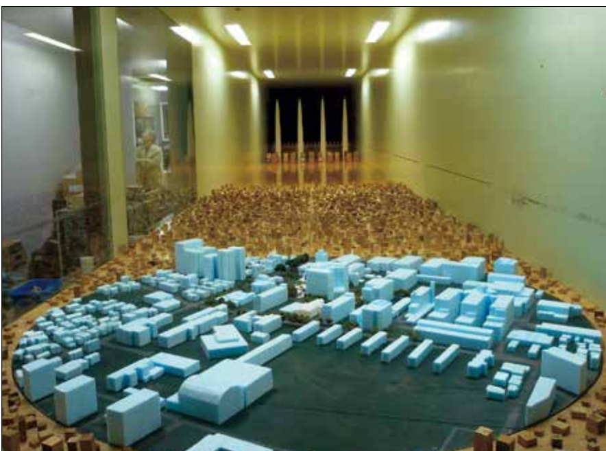
Picture 2: Wind tunnel testing used in comparative evaluation
