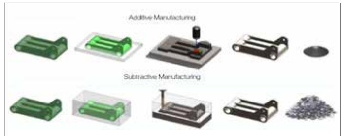
Figure 4: Comparison of Additive and Subtractive Manufacturing
