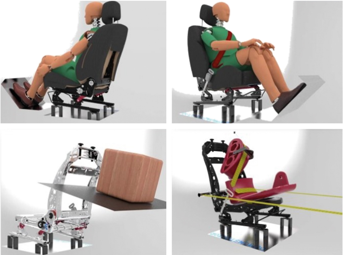
Fig 1: Four severe seat load cases at high speeds, top left is a front crash, top right is a rear crash, bottom left is a 18kg luggage crash, and bottom right is seatbelt anchorage test.
