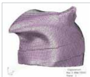
Mesh generated in Patran using the Marc Hex Mesher
