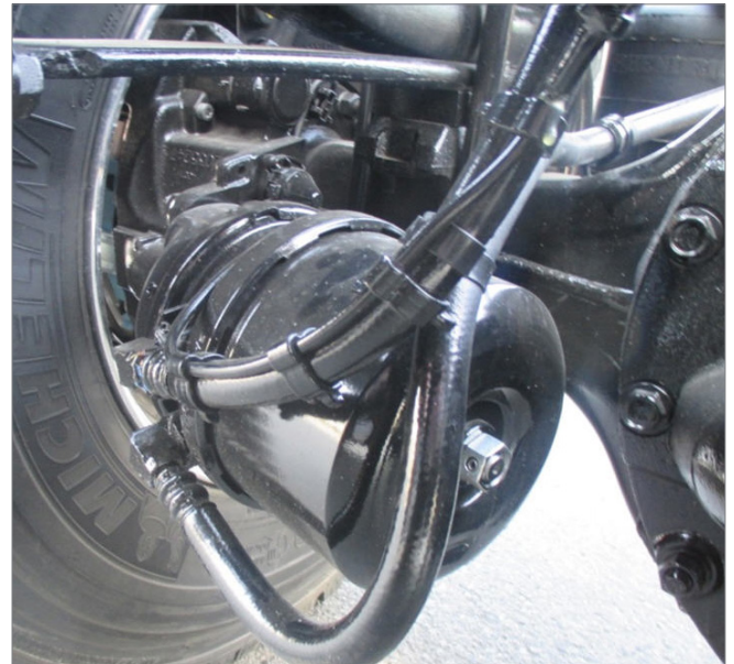
11 hoses are routed in a typical tandem suspension
