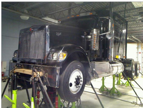
Hose routing configurations are evaluated on a test rig
