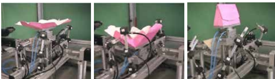
Figure 4. D-RAPS robot in operation folding carton
