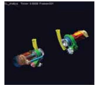
Figure 4: Adams model of DC gear motors
