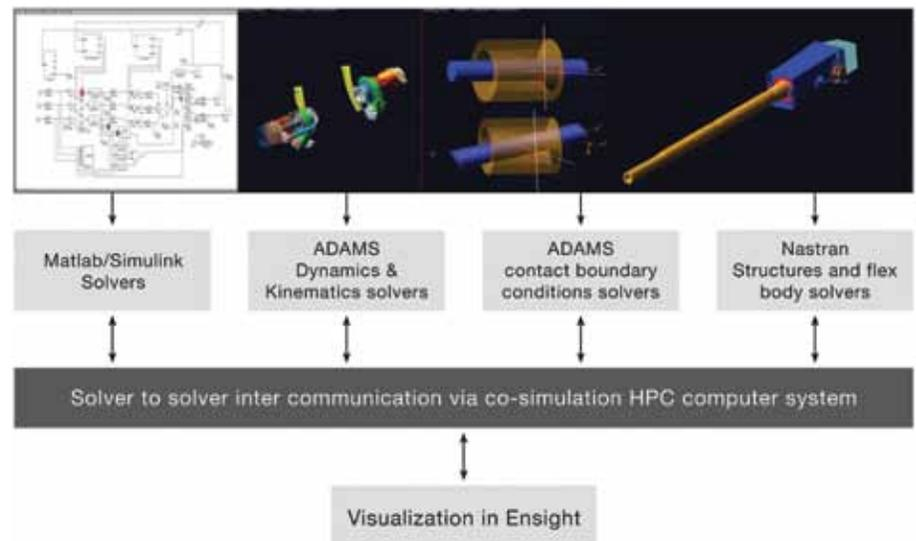
Figure 1: Overview of co-simulation process
