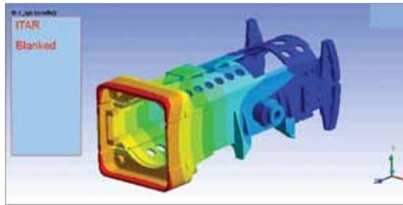
Figure 3: First modal frequency for cradle is outside bandwidth of interest so it was modeled as rigid body
