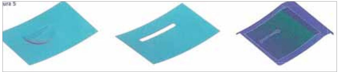
Figure 4: The image on the left shows a finite element model of the contact surface of the initial design of the stamping die. The center image shows the finite element model of the initial design of the flat panel geometry. The image on the right shows the models of the tool and material combined with the contact algorithm.
