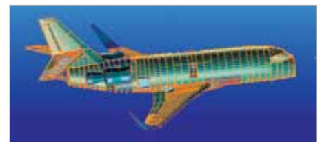
TLG customer aircraft modification. TLG performed the complete static & dynamic loads, and flutter certification analyses using MSC Nastran.
