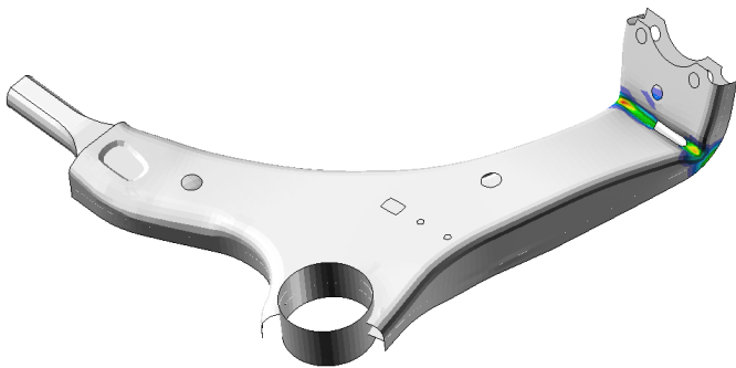
Elasto-plastic simulation of an automotive link arm
