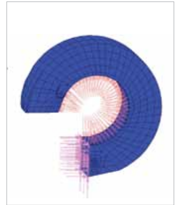
Finger sub-assembly Surface Pressure Load generating Tension & Bending
