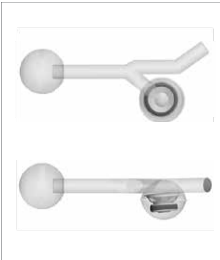
Exhaust line with Active Noise Cancellation system: Top view and Side view
