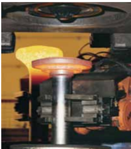
The part is shaped firstly by upsetting (in the background).
